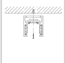
step 3.: Fit magnetic profile onto mounting surface with self-tapping screws.
