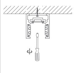
step 4.: Put the end caps to the profile and secure with the screws.
