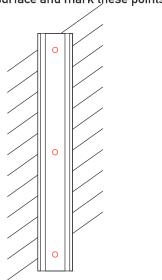
step 2.: Drill the points and insert dowels into mounting surface. Touch profile on the mounting surface and align the holes.
