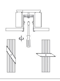
step 5.: Keep screwing to lock the fixation part with the ceiling. Connect the terminal block according the electrical instructions.
