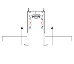
**step 4.:** Screw the fixation parts in order to open the tool.
